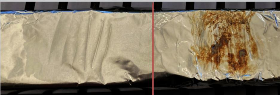
Left: GEO WWF-U300 > burns without residues and has a clear sliding effect at 300°C.
