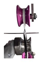
In the process zones of this wiping system, a woven textile tape wraps around the material surface. The continuously adjustable transport of the textile tape ensures that there is always a clean wiping tape in contact with the material to be cleaned.
