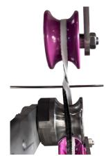
In the process zones of this wiping system, a woven textile tape wraps around the material surface. The conadjustable tinuously transport of the textile tape ensures that there is always a clean wiping tape in contact with the material to be cleaned.
