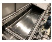
guided in parallel above the ultrasonic units in a tank flooded with cleaning medium. If only a few wires are routed closely together, GEO's tubular reactor can be used.
