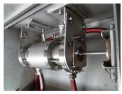
GEO uses compact highpressure nozzles specially designed for industrial continuous profile cleaning in its high-pressure cleaning systems. The nozzles apply a tem-
