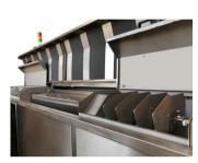
Powerful ultrasonic modules, high pressure- / and steam nozzles, integrated in space-saving inline equipment with liquid management, guarantee outstanding re-
