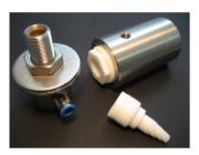
A surface is dried by an airstream, which is lead through a helical teflon body inside the nozzle. The airstream is accelerated, pushed into rotation and blown against the
