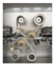
The KFP system is designed to remove misprints on cables in a continuous process. For this purpose, the cable is exposed to a suitable solvent and mechanically wiped in two steps by nonwoven tapes.
