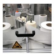
The solvent required to remove the labeling is applied to the cable from a container in metered quantities, distributed evenly by static brushes, and then picked up or wiped off again by pairs of nonwoven tapes arranged in an offset pattern. These tapes are wound up by
