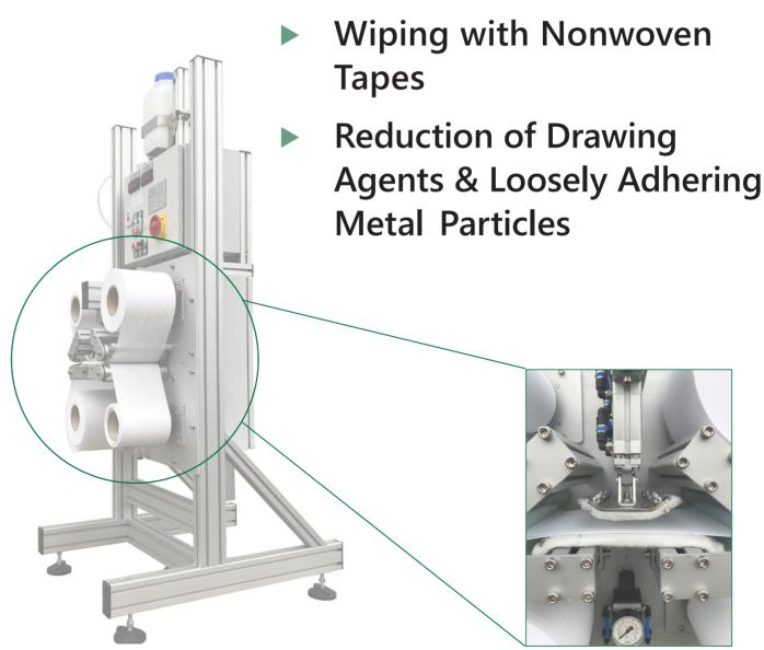
PWW - Wiping with non-woven fabric. Ideal for cleaning thin and / or multiple, parallel wires and narrow belts, dry or wet. Perfect for a wide range of cleaning applications
