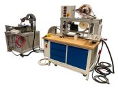
The design of the WWTE measuring device for welding wires is based on the fact that the quality of a weld depends decisively on the quality of the welding
