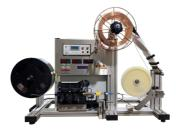
Like the WWTE measuring device, the WWTE I table-top device is used for quality assurance of welding wires. In contrast to the WWTE, testing of the wire properties with
