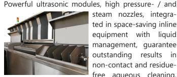
steam nozzles, integrated in space-saving inline equipment with liquid management, guarantee outstanding results in non-contact and residuefree aqueous cleaning,
