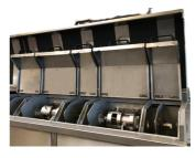
Similar to our ultrasonic systems, the material passes through various treatment zones. The ready-to-use units are equipped with one or more heatable, insulated tanks. A
