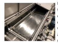
immersible Ultrasonic transducers are the first choice for multi-wire cleaning. In this case, the wires are guided in parallel above the ultrasonic units in a tank flooded
