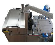
Steam is another option for generating clean, oilfree material surfaces. The nozzles used in the process zone are used singly or in combination with a high-pressure nozzle.
