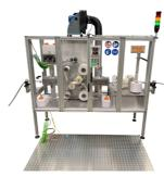
via doors. An exhaust channel with explosion-proof fan keeps the work area free of vapors. Further explosion protection measures complete the equipment.
