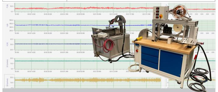
The standard WWTE system is operated with commercially available MIG / MAG welding equipment with a maximum welding current of 500 A (water cooling required). Without interruption, the maximum welding time is 10 minutes at 500 A.
